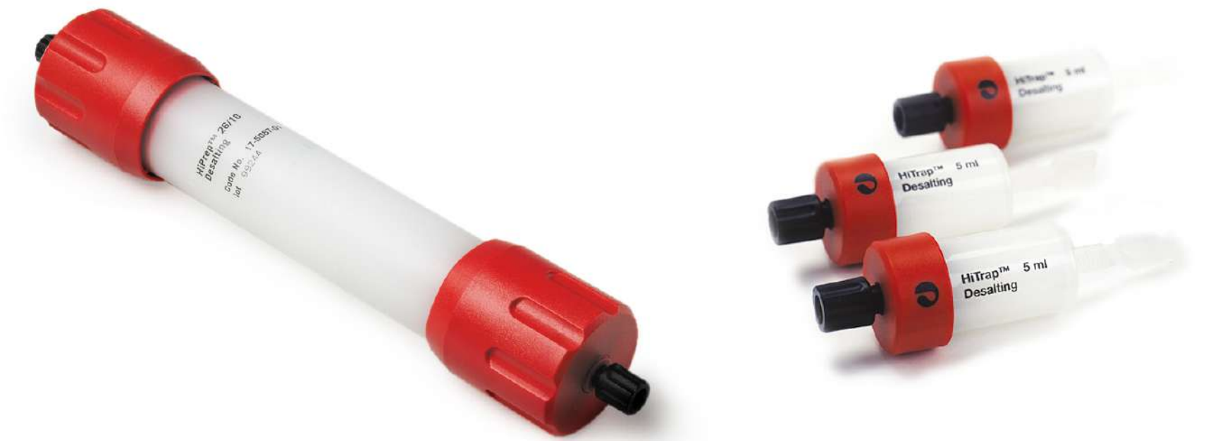
Fig 5.6. Prepacked Sephadex G-25 columns: left HiPrep 26/10 Desalting, right HiTrap Desalting.
