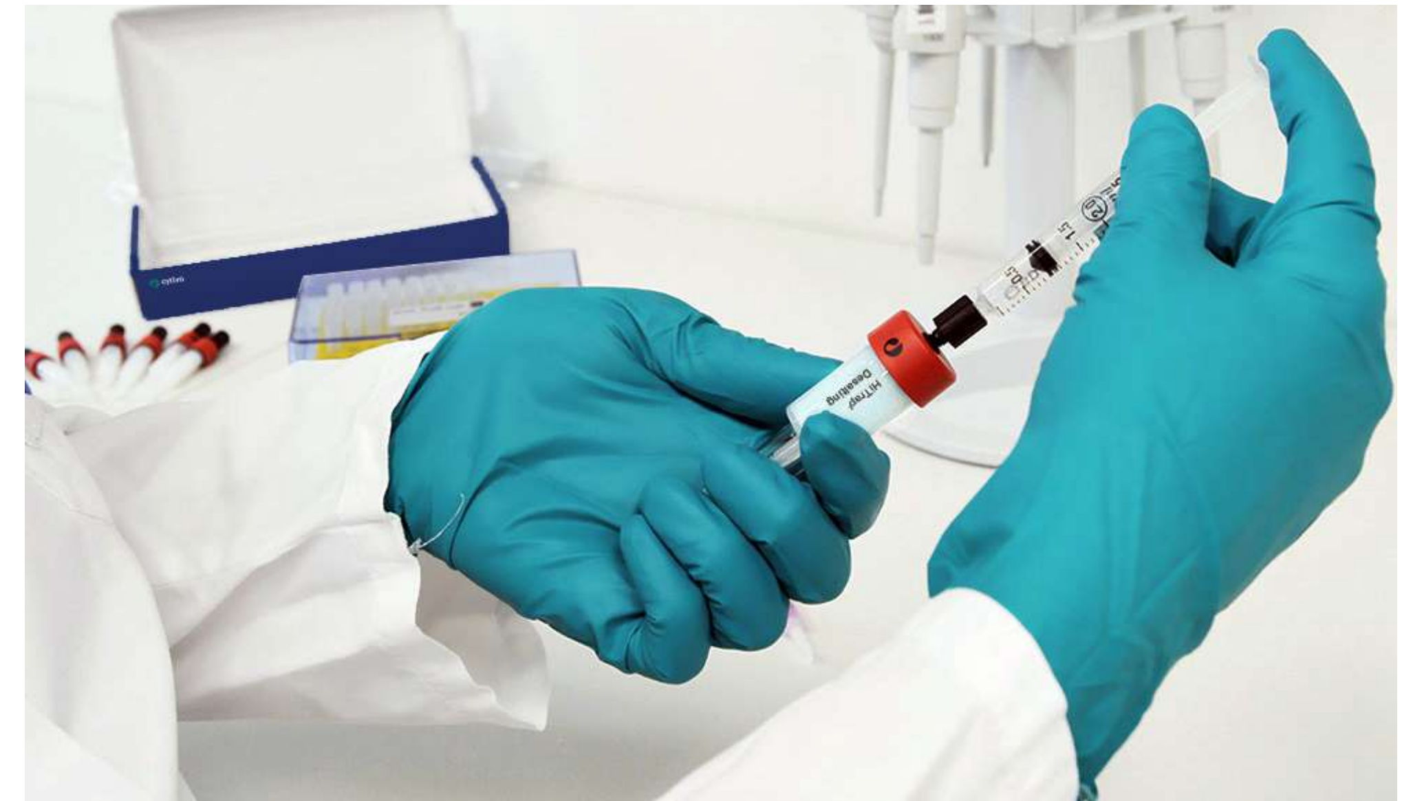
Fig 5.8. HiTrap Desalting column operated by syringe.
