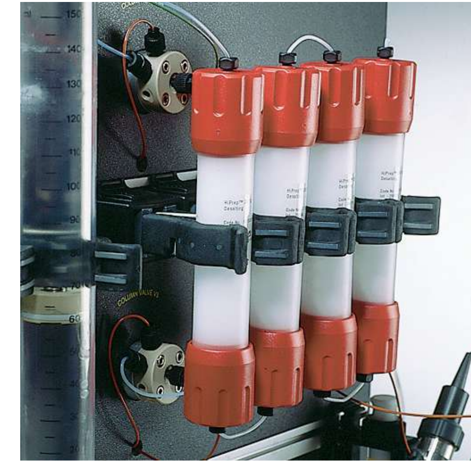
Fig 5.9. Four HiPrep 26/10 Desalting columns connected in series.
